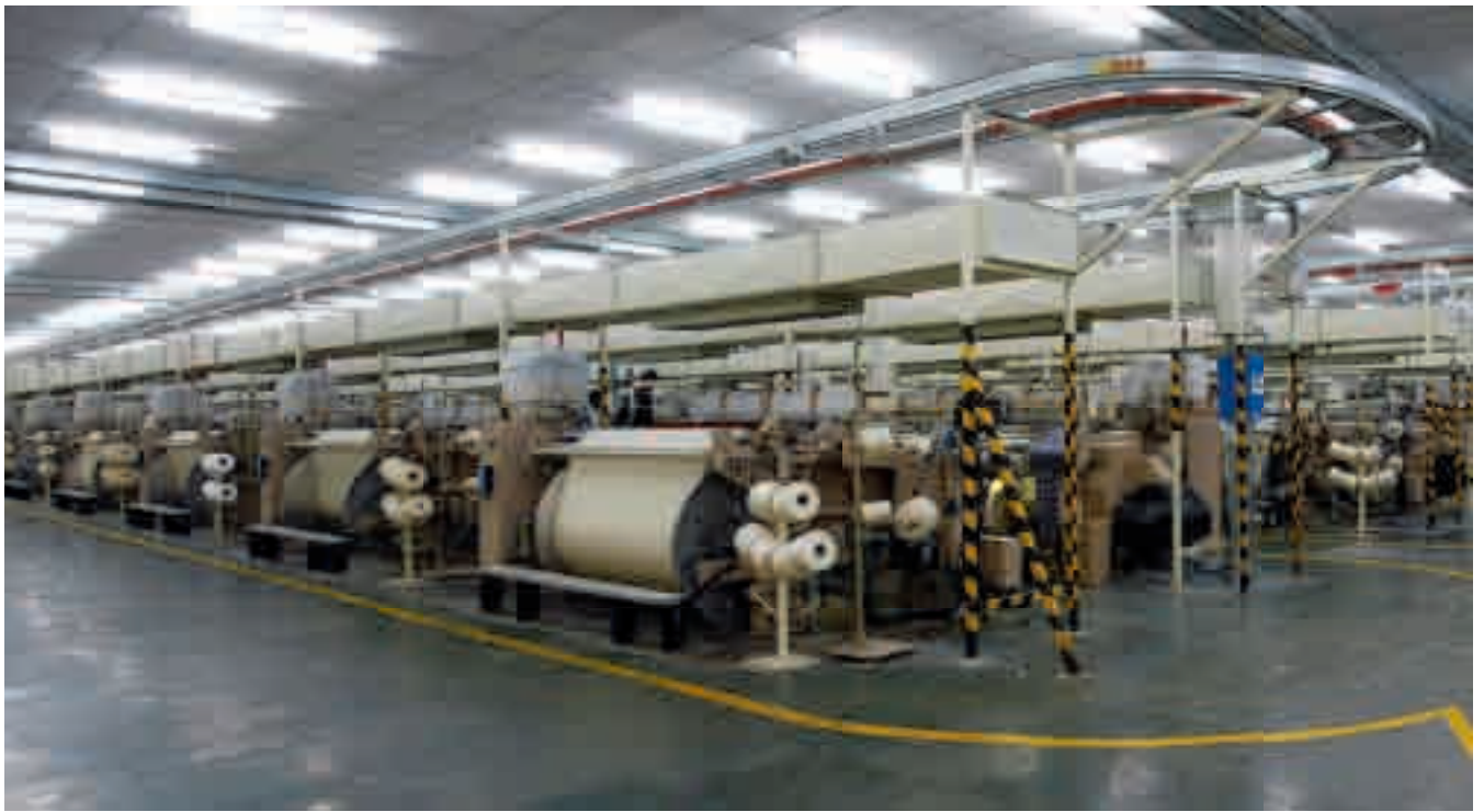
A panoramic view of the state-of- the art weaving loom machine producing grey cotton fabric at the integrated textile unit of the company at Vardhman Fabrics, Budhni
