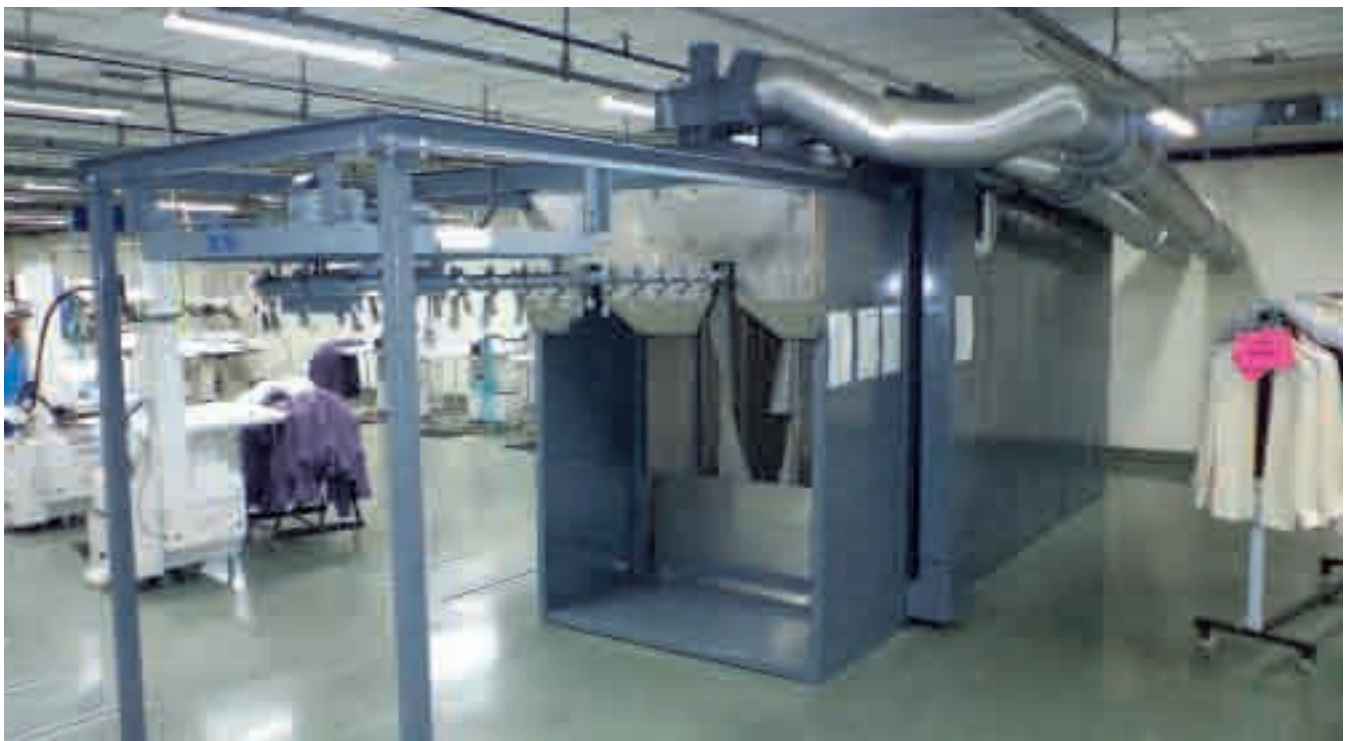
Baking machine in operation for making S.S.P (Wrinkle free) shirts at one of the subsidiaries of the Company- Vardhman Nisshinbo Garments Company Limited, Ludhiana.
